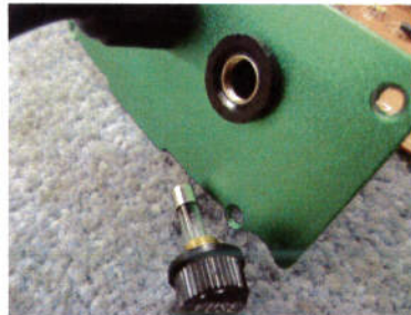
Shows live screw thread accessible by hand.
