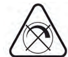
Fig 16. Symbol that lamp is not suitable for use with a dimmer switch.
