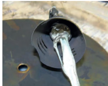
Fig 8. Luminaire after fatal fire. The remains of the plastic body of the lamp can be seen protruding from the body of the luminaire. Image courtesy of London Fire Brigade.
