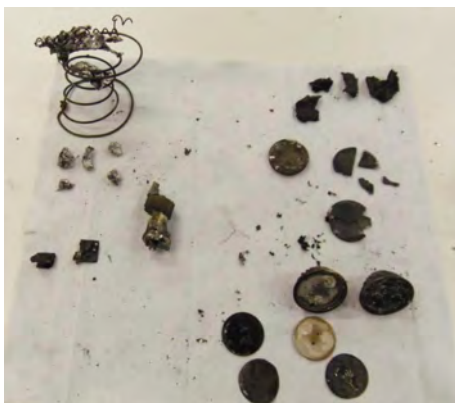
Fig 7. Parts of damaged LED lights found within the remnants of a bed deemed to be the source of fire that resulted in a fatality. Note the remains of an aluminium heatsink melted onto one of the mattress springs. Image courtesy of London Fire Brigade.
