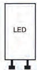
Fig 11. LED replacement starter marking
