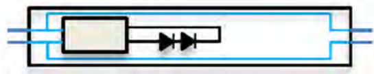
Fig 13. Simplified circuit diagram of one type of double capped LED linear lamp available for purchase. With this configuration, if the lamp is installed into a luminaire providing both line and neutral to one end of the lamp, the pins at one end of tube will be hazardous-live when the pins at other end of tube are engaged in the lampholder whilst circuit is still energised. See also Figs 14 and 15.
