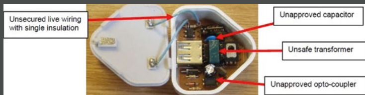
△ Detail of counterfeit interior, provided by Nemko Ltd.
