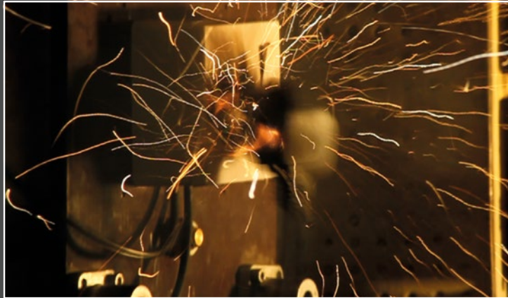
△ An image taken during the testing, showing one of the plugs exploding away from the socket outlet as a result of the catastrophic failure of the fuse.
