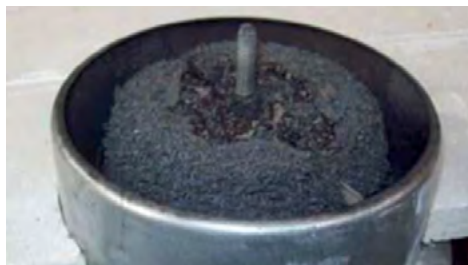
Fire rated Ceiling Air Valve sealed after a fire Photos courtesy of Tenmat Ltd.
