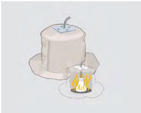
Typical fire hood for a downlighter.
