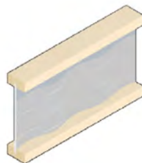
Steel webbed, timber 'I' beams; consisting of corrugated steel webs with timber top and bottom chords.
