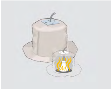
Typical fire hood for a downlighter.
