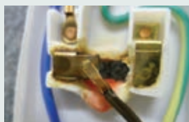
Fuse holder completely melted due to overheating
