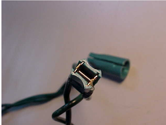
Figure 12 “chip” in situ between contacts
