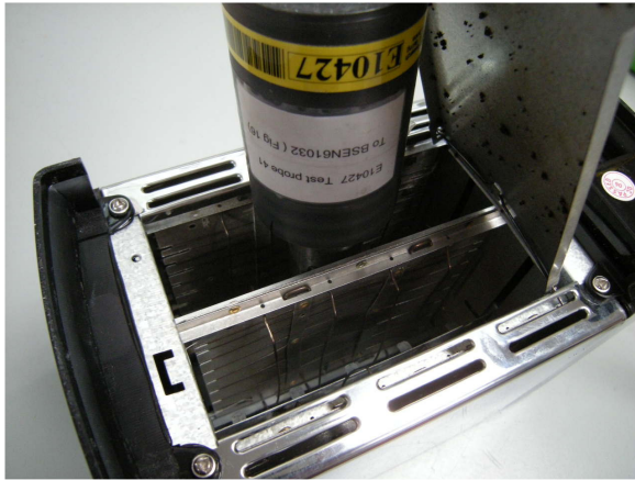
Figure 7 Application of test probe
