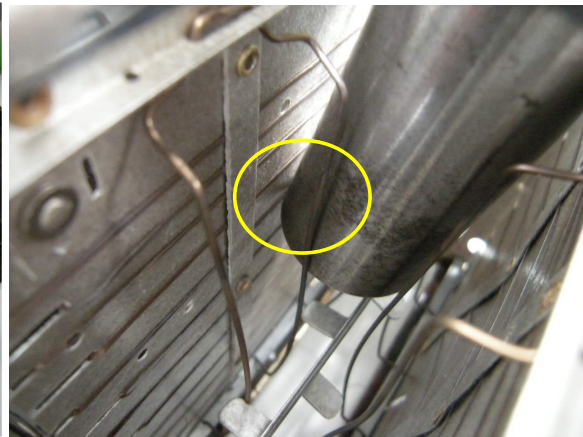
Figure 8 Test probe touching live parts
