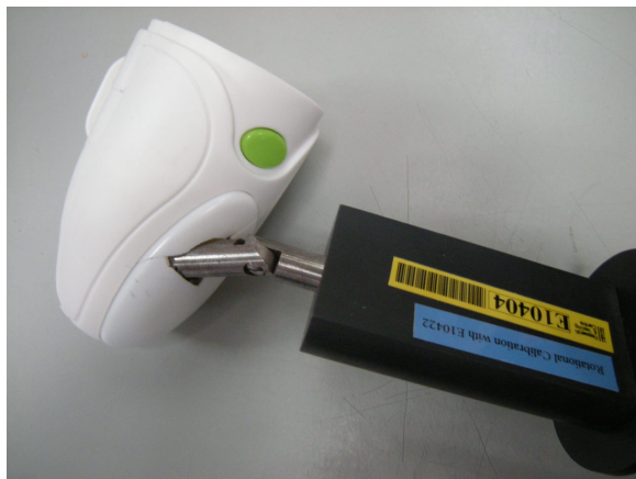
Figure 3 Access to live parts with test finger
