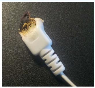
Example: Charger pin damaged because of using wrong device
