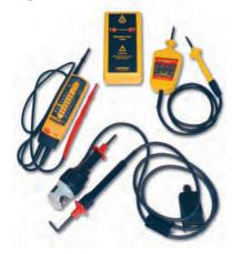
The test lamp or voltage detector should be proved to be working on a compatible proprietary proving unit, or a known live source, or an in-built test function before and after use.
