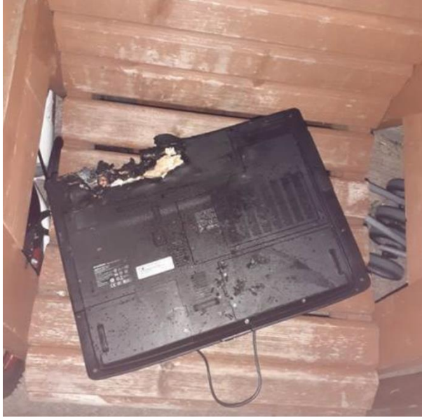
Damage to the laptop caused by the battery.
