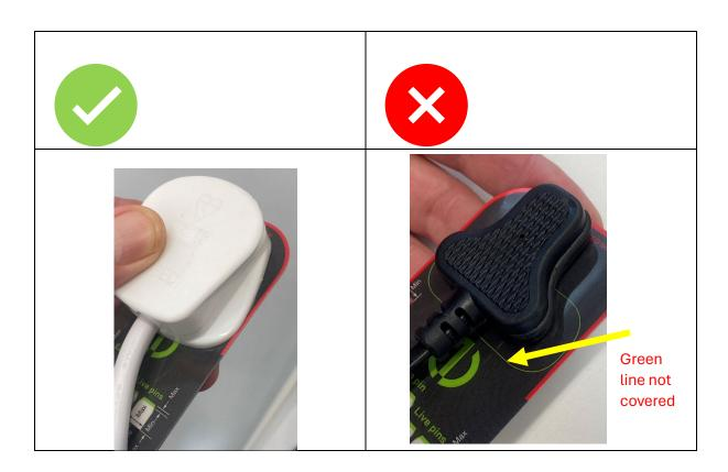
(5) Pin lengths and widths must also be checked; pin lengths must be within the GREEN ZONE, pin widths must not exceed that shown on the diagram and the Insulation on the live pins must be within the BLACK zone.
