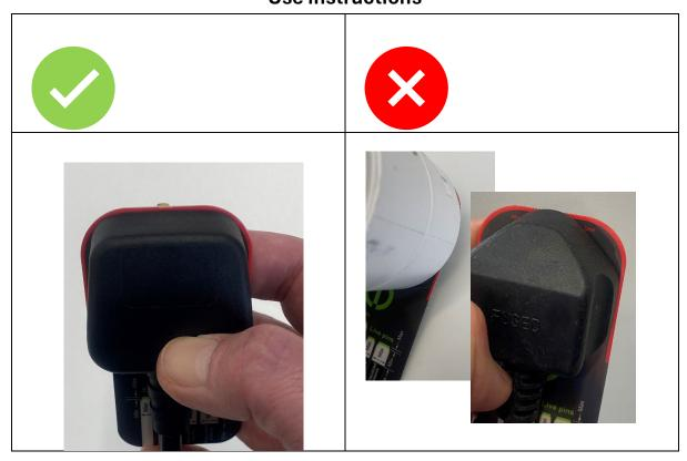
(4) With the plug fully inserted into the plug checker, all of the GREEN line must not be visible.
